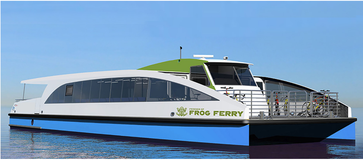
The double-hulled electric catamaran chosen for the Frog Ferry pilot project could carry 70 passengers at about 30 mph.
