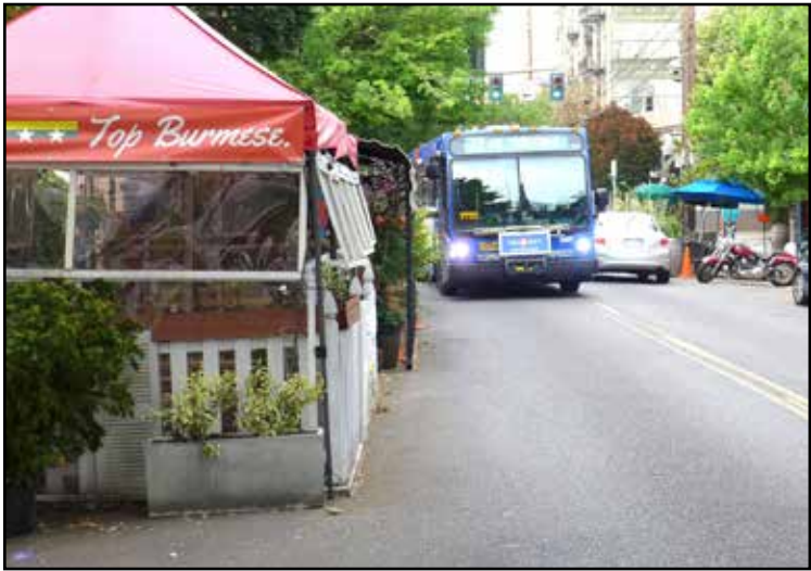
Shelters along both sides of Northwest 21st Avenue force buses to cross the centerline. Photo by Wesley Mahan
